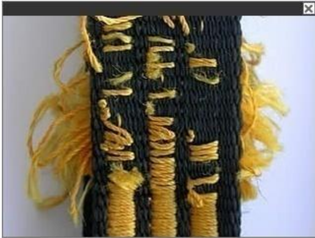
Ripped energy absorber (To Reject)
